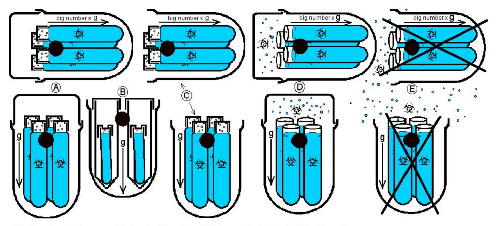
Infectious Aerosol Management During Centrifugation with Various Swinging-Bucket Rotor Assemblies
