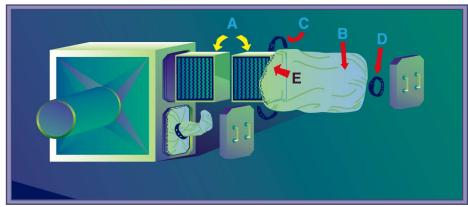
This shows the BIBO filter enclosure with (A) filters, (B) bag, (C) safety straps, (D) cinching straps, and (E) shock cord in the mouth of the PVC bag restricts the bag around the second rib of the housing lip.
