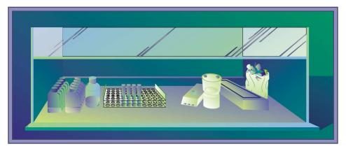
Working "Clean to Dirty" in a Class II BSC. Clean cultures (left) can be inoculated (center); contaminated pipettes can be discarded in the shallow pan and other contaminated materials can be placed in the biohazard bag (right). Reverse the arrangment for left-handed persons.
