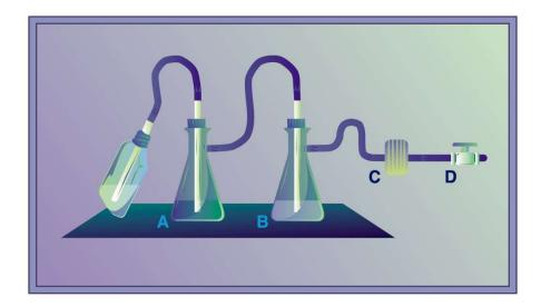
The left suction flask (A) is used to collect the contaminated fluids into a suitable decontamination solution; the right flask (B) serves as a fluid overflow collection vessel. A glass sparger in flask B minimizes splatter. An in-line HEPA filter (C) is used to protect the vacuum system (D) from aerosolized microorganisms.
